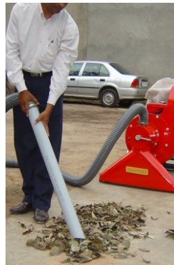
Bulk Materials' removal with flexible hose
