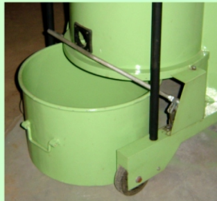
Foot operated Lift & Lock Mechanism for the container
